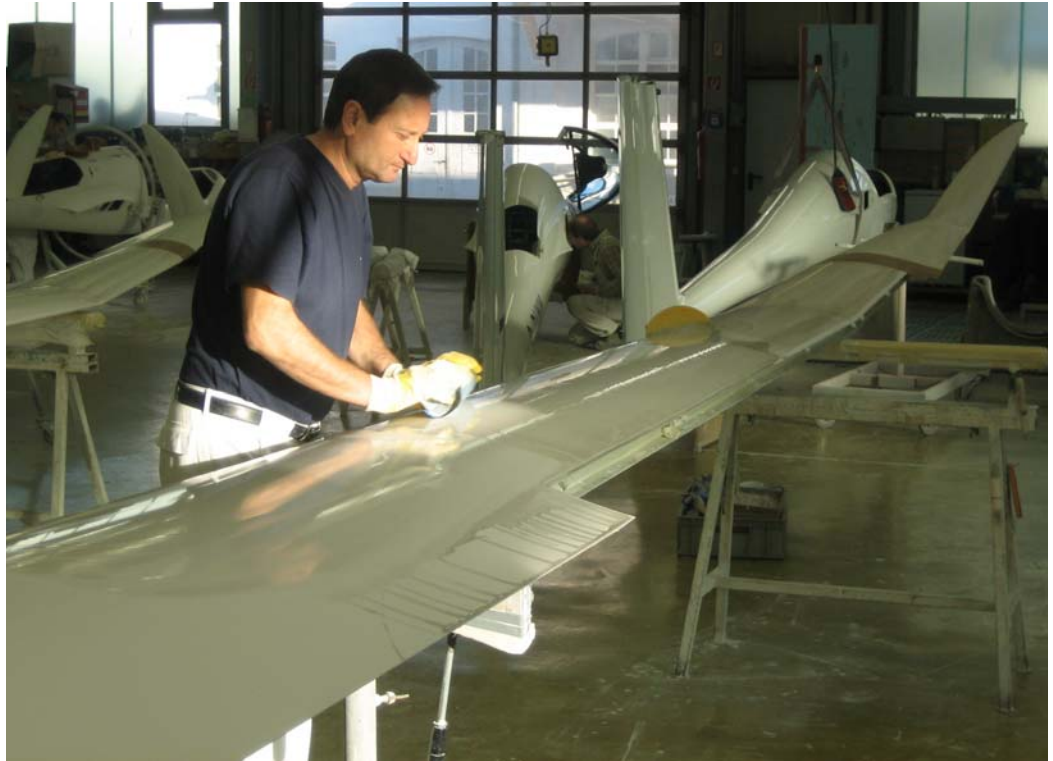
A craftsman meticulously sands the wings of my new glider in Germany.
